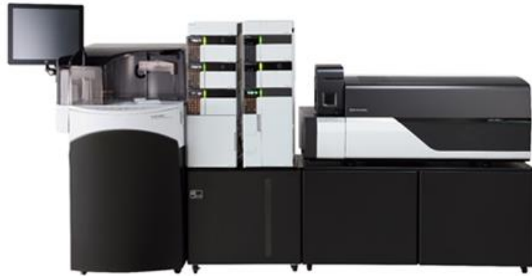
Fig.1 Automated and Integrated system CLAM-2000 coupled to LCMS-8060
